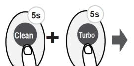
Press together **Clean** button and **Turbo** button at the same time more than 5 seconds to activate Lock function. All buttons will not response except pressing these two buttons for two seconds again to disable locking.
