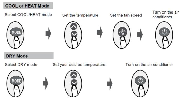
NOTE: In DRY mode, fan speed can not be set since it has already been automatically controlled.
