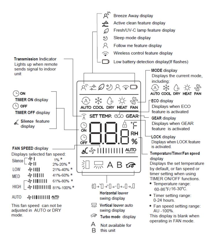
**Note:** All indicators shown in the figure are for the purpose of clear presentation. But during the actual operation, only the relative function signs are shown on the display window.
