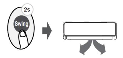
Keep pressing this button more than 2 seconds, the vertical louver swing function is activated. (For the units with vertical louver swing feature)
