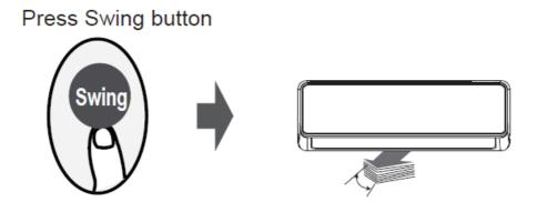
The horizontal louver will swing up and down automatically when pressing Swing button. Press again to make it stop.
