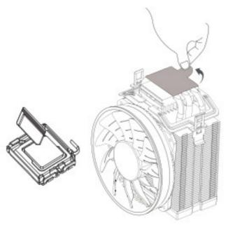
STEP 2: Install the CPU then attach the clips to the AMD motherboard brackets
