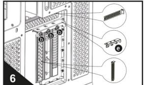
**Note:** To install the graphics card in a vertical position, a GPU riser cable is required (not included). It is recommended to use a GPU riser cable of at least 300 mm in length, such as the Mars gaming MCAPCIE 40 model.
