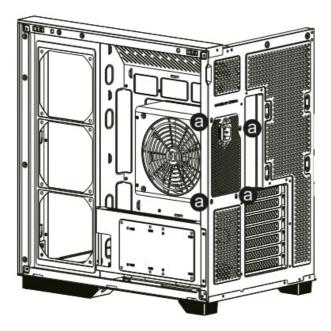
3. **Motherboard installation:** Install an ATX/MicroATX/Minil TX motherboard and screw the screws in the position corresponding to your motherboard.
