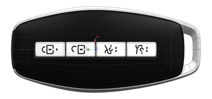
The UK1 has four keys: Open, Close, Trunk and Frunk. On each button press, it initiates the communication to the MUB1 and the range measurement process.
