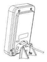
Before use, the Buddy must be assembled onto its stand and the USB connector plugged into the back of the unit.
