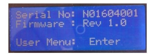
Press ENTER to view the programming menu. Use the UP and DOWN keys to scroll through and ENTER to select an option. A cursor indicates the option available to select.
