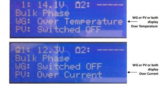
When the condition subsides the normal display is automatically resumed except in the case of PV over current. See below.
