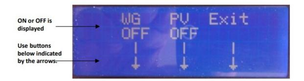
Toggle the UP and DOWN buttons to change between ON and OFF. Press ENTER to Exit. Note that when switching WG to OFF the controller enters a soft stall routine, this slowly applies the stall to decelerate the turbine. During this routine, the following is displayed and when complete the display returns to the programming menu.
