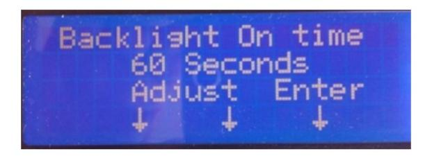
Adjust the seconds using the UP and DOWN buttons to the desired duration, one press adjusts one second. Press ENTER to save this time to non volatile memory and return to the programming menu.
