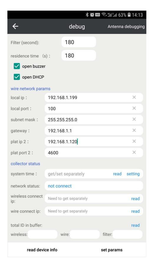
After set params, open the server demo and input the IP and port. Click Start button, reader will output data to server demo automatically.
