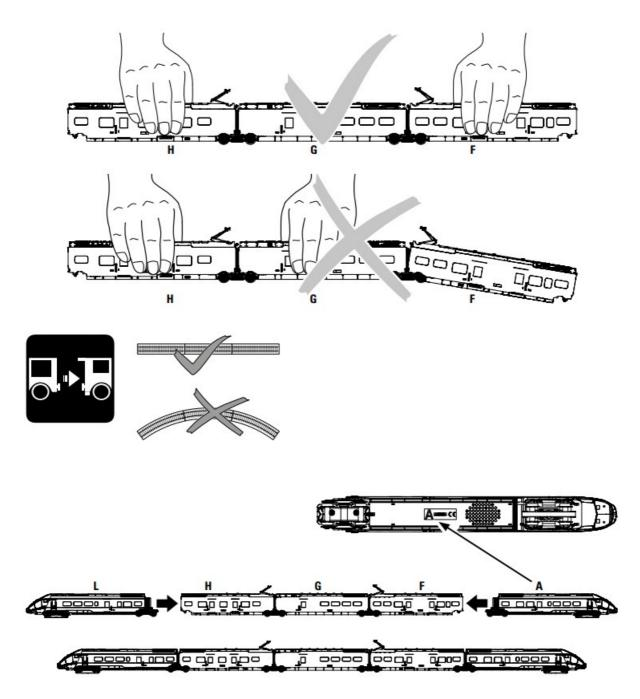
To uncouple, lift gently, and use the uncoupling tool included with this model to unlock at the car floor.
