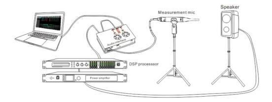
Using third party software to set FIR magnitude and phase **Step 1:** measure phase curve of speaker in Smaart V7
