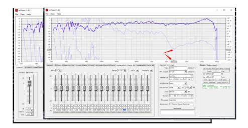
Step 4: adjust phase EQ or any other parameter in software, to match a linear phase for speaker
