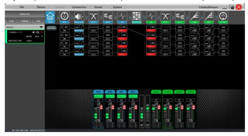
Open Mconsole software, user can choose an input channel or output channel as needed, such as FIR in output channel, it will show a FIR function window.
