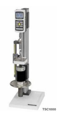
The TSC1000 is a rugged stand for heavy duty testing requirements requiring fine position control without back driving. Hand wheel operation allows the operator to produce gradual and repeatable force during testing. Modular design allows for the gauge mounting plate and housing to be moved along the length of the column. Removable base (TSC1000) or mounting legs (TSC1000H) allow for a range of custom mounting configurations.
