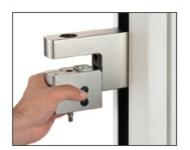
Series FS05 force sensors mount directly to the crosshead. Match the gold-plated pads on the top surface of the load cell block with the pins in the underside of the crosshead, as shown at left.
