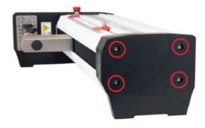
The end cap is shipped in a separate box within the main box for the Model F505H test frame. Line it up with the right end of the column, then install with the four included screws, as shown at left.
