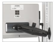
Tighten the screw that joins the crosshead to the force sensor. Optionally cover the screw head with the included black plastic cap.
