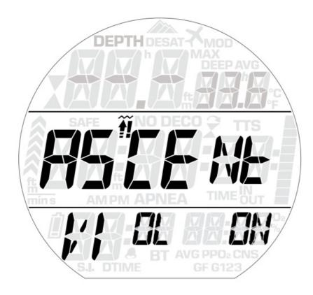
If the ascent rate exceeds 120% of the allowed value over a depth change of more than 20m/66ft, due to the potential of harmful bubble formation, Puck 4 locks the computer for 24 hours in order to prevent you from diving again. In this menu, you have the option to disable the locking up of the computer in the event of an uncontrolled ascent.
