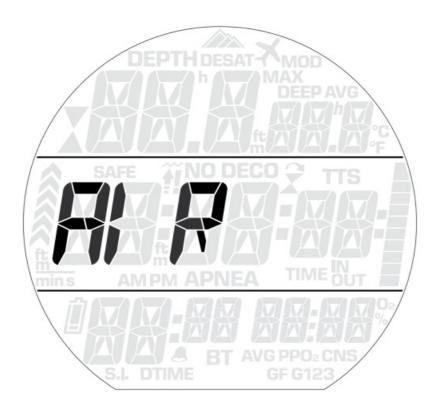
When selecting NItROX, you are taken to a submenu in which you can define the percentage of oxygen in the mixture (O2%) and the maximum value of oxygen partial pressure (ppO2max) for up to three breathing mixes. The maximum possible value for the ppO2max is 1.6bar. Most training agencies recommend not to exceed a value of 1.4bar.
