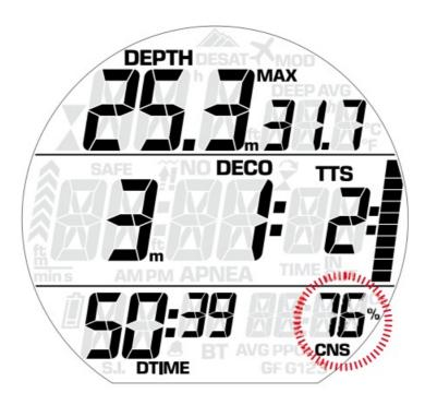
If the oxygen toxicity level reaches 75%, ascend to shallower depth to decrease oxygen loading and consider terminating the dive.
