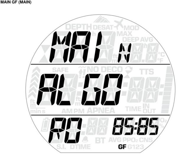
This is where you set the conservatism level of the ZH-L16C algorithm via gradient factors. We use Bühlmann's original values reduced by 15% as a starting point, and you can make the algorithm more conservative from there. There are four predefined sets of gradient factors with increasing conservatism from R0 (85/85) to R3 (50/60). You can also enter the GF low and GF high values directly via the CUStOM setting. The default value is R0 (85/85).
