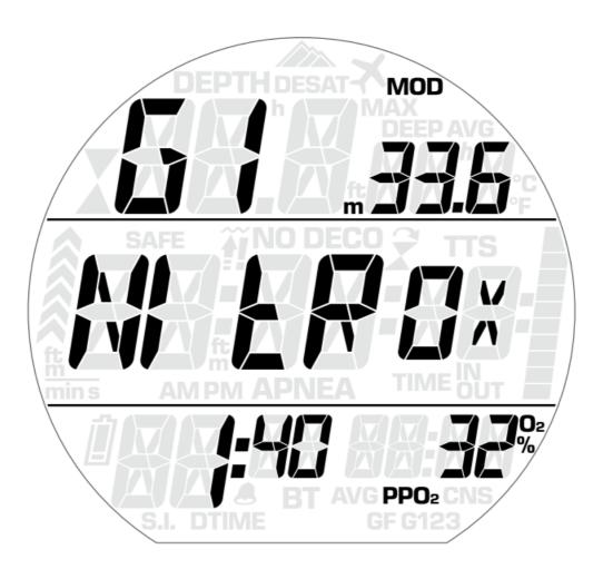
Once inside this menu, press the button to change the O2%, and watch how this affects the maximum operating depth (MOD). Then press and hold the button to move on to the ppO2max and press the button to change the value, again noticing how this affects the MOD. Press and hold the button to save and exit the menu. At this point
