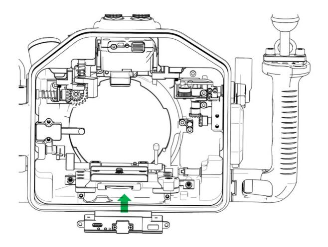
For the Wireless Shutter Module: Insert the shutter release cable, then install the module into the bottom slot of the housing quick-release plate.
