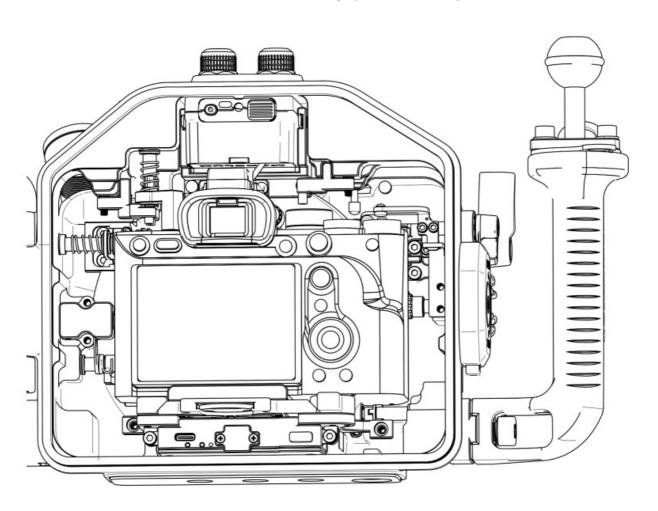
Secure the module with screws. Insert the shutter release cable into the camera and then install the camera into the housing.
