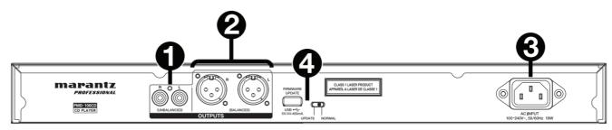
**Outputs (unbalanced RCA):** These outputs send the audio signals from a CD, USB device (mass storage class), and device connected to the Aux-In. Use RCA cables to connect these outputs to external speakers, sound systems, etc. See **Setup** for more information.
