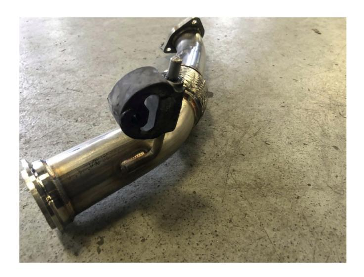
**Step 9**Slide the front half of the front pipe into place and install it on the hanger
