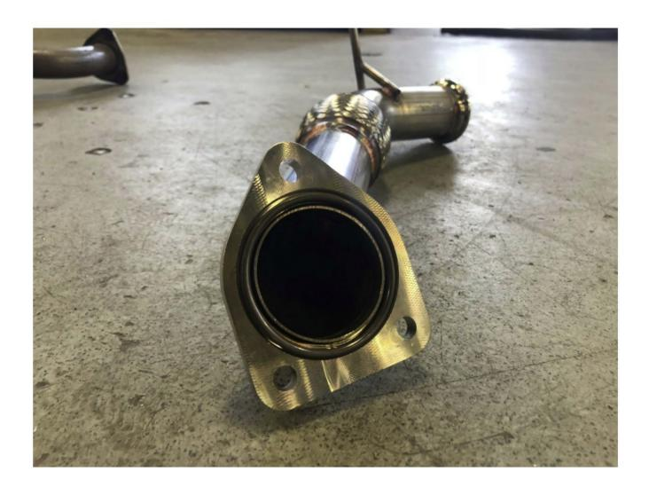
**Step 8**Remove rubber hanger off your old front pipe and install it onto your new front pipe use of silicone grease will make this much easier
