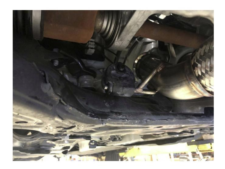
**Step 10**Reinstall nuts onto front pipe to downpipe flange
