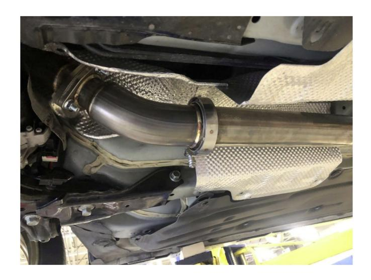
**Step 17**Startup and check for leaks, once satisfied reinstall splash shield
