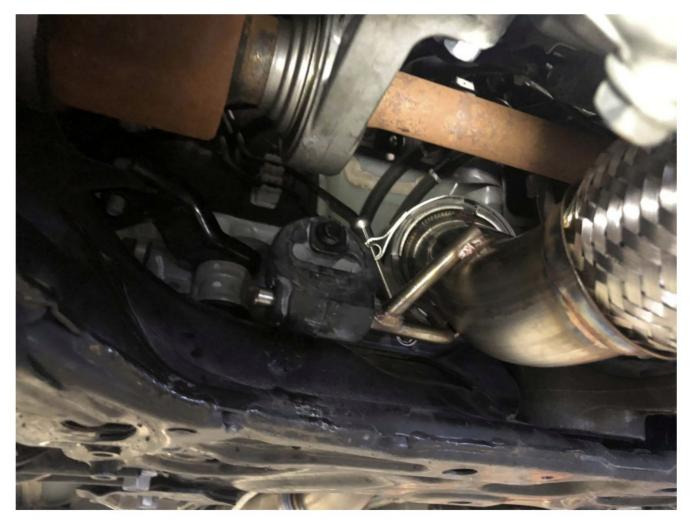
**Step 12**Install rear section to front pipe, secure it LOOSELY with the vband clamp
