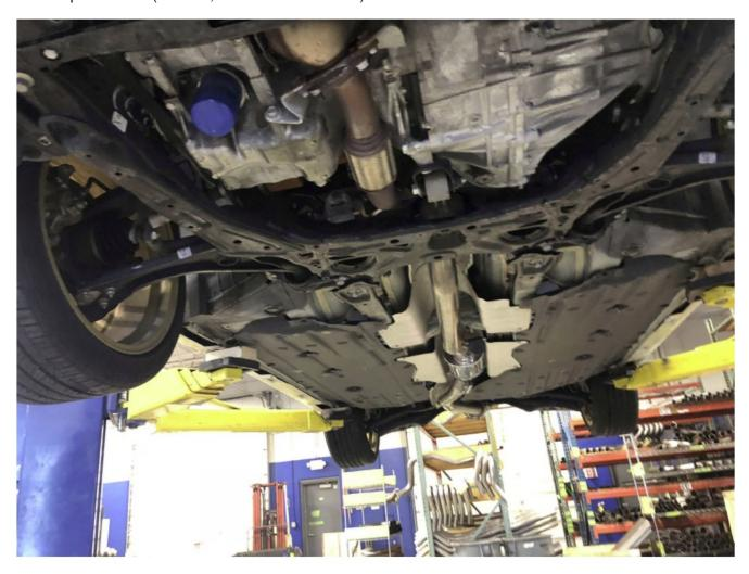
**Step 2**Remove 3 downpipe nuts (the studs may pull out, this is fine)
