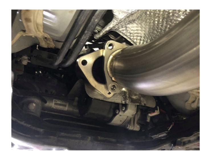
**Step 14**Install included 3 bolt gasket and hardware, secure the front pipe to the catback
