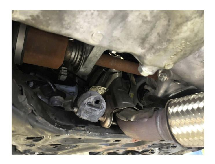
**Step 5**Remove 6 10mm bolts holding the heat shield on and slide it back
