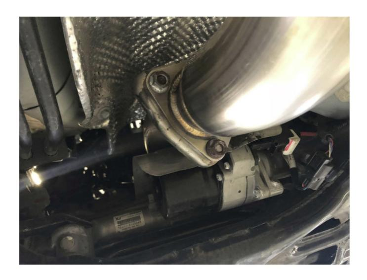
**Step 4** Remove front pipe from hanger
