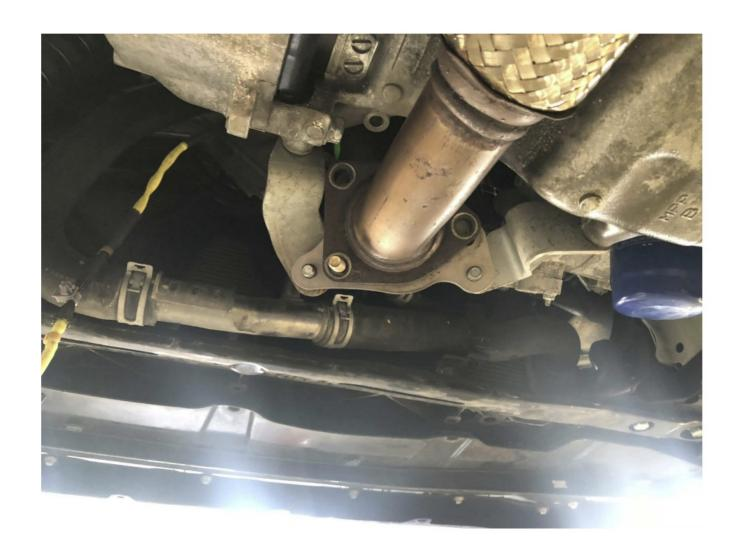
**Step 3** Remove 3 front pipe to cat back nuts
