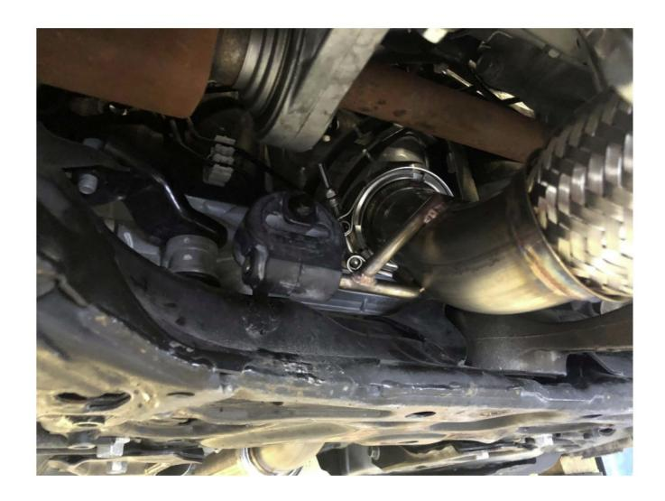
Step 16 Reinstall heat shield
