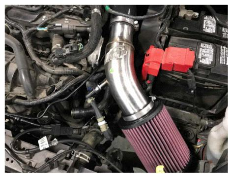
Connect the hose you installed earlier onto the intake, plug the maf sensor in and ensure all worm clamps are tight
