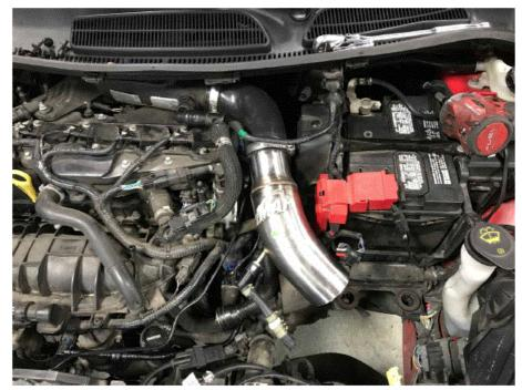
Install the MAF sensor onto the intake pipe, then install the intake onto the vehicle. secure the intake to the engine via the stud located under the vacuum pump. You will need to remove the nut and reuse it
