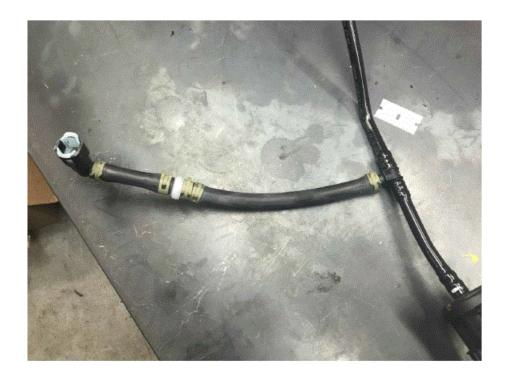
If 2016+ Use a razor blade to cut a slit in the hose a the T fittings, this would be the hose you disconnected earlier. Then install the included (and pictured) hose onto the T fitting
