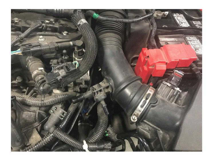
If 2016+ Remove 2 lines attached to the valve connected to the intake tube. The connectors are secured by a clip that needs to be lifted up on both sides to slide up, this will allow you to remove the fittings from the valve
