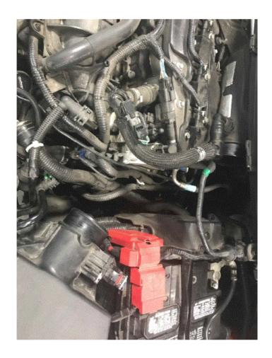
Remove intake tube, it should compress and slide out easily
