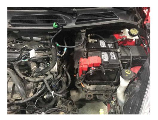
Remove intake filter box, you will need to unclip the intake snorkel and then the entire box will lift up and out with some force
