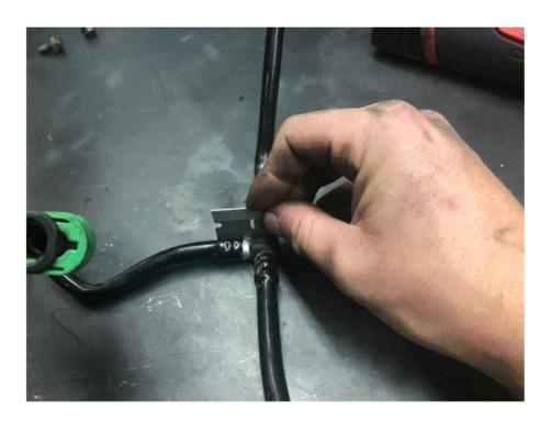
If 2016+ Use a razor blade to cut a slit in the hose a the T fittings, this would be the hose you disconnected earlier. Then install the included (and pictured) hose onto the T fitting
