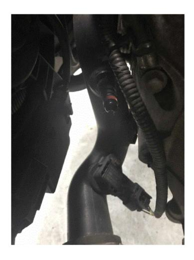
If 2016 + Removed the hose connected to the lower charge pipe and cap the charge pipe with the included fitting (as pictured)
