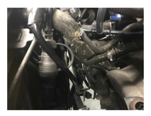
If 2016 + Removed the hose connected to the lower charge pipe and cap the charge pipe with the included fitting (as pictured)
