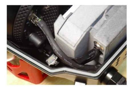
14. Hybrid cable only: Replace the original battery tray with the DC converter tray and connect the power lead from the hybrid bulkhead.
