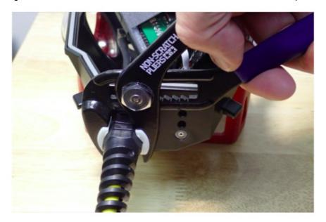
**Notes** for hybrid cable installation: The hybrid cable features a waterproof connector, which can be detached from the bulkhead. Please make sure the cable is detached from the bulkhead during installation.
