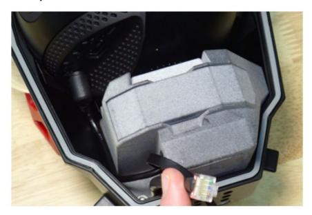
13. Now connect the newly installed cable to the camera. Fold the flat housing ethernet cable that comes with the internal tray away, it is not used in this configuration.
