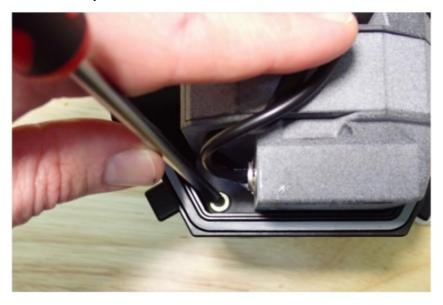
3. Place the tray slightly to the side in the housing. Keep it upright so that the bolt doesn't fall out.
