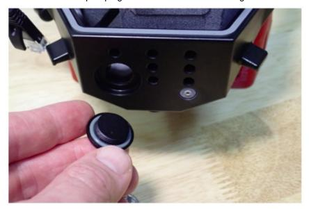
2. Remove the bolt securing the tray to the housing with a 4mm hex key or driver. You do not need to remove the bolt from the tray.
