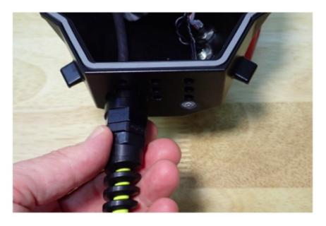
7. Tighten the bulkhead connector with a 22mm wrench of non-scratch pliers.
