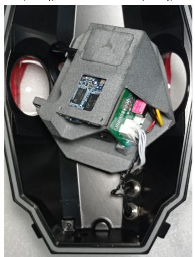
3. Confirm that all three XH connectors are seated properly and that no individual leads are exposed.
