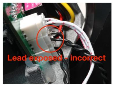
5. To fix the faulty connector, remove it from the socket and push the pin fully into the connector housing. Then reseat the connector.
