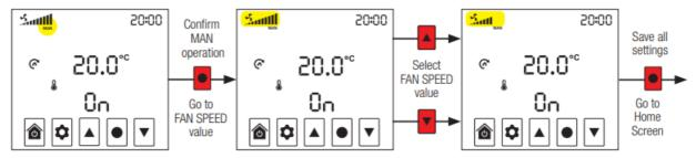
Fan speed will remain constant at the speed set. If system is in BOOST mode, the fan will operate at the speed set for that mode.
