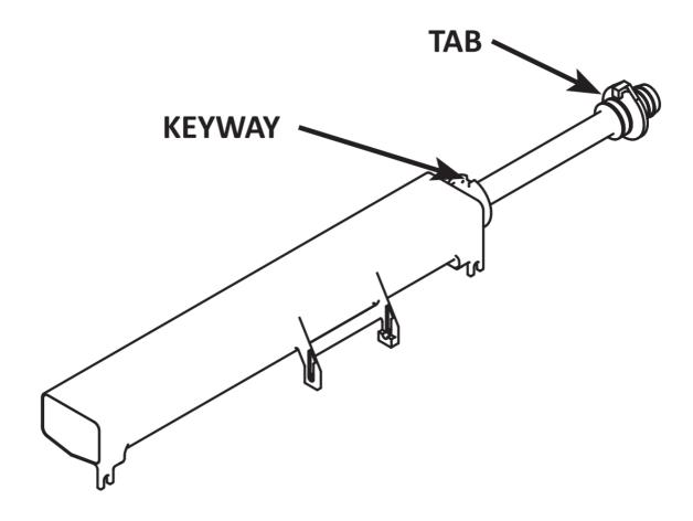
Water Distribution Tube Disassembly F. Remove the Float Valve.
