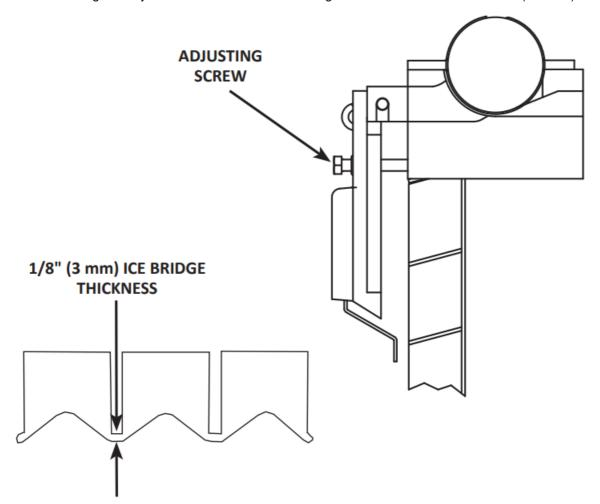
Make sure the ice thickness probe wire and the bracket do not restrict movement of the probe.
