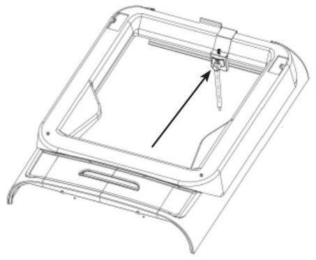
6. Secure bracket to adapter using screw provided.
