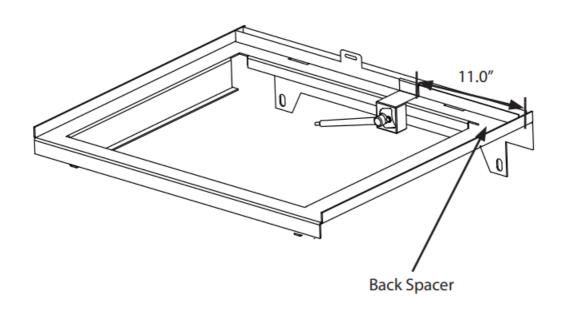
6. Route thermistor wire out towards the back of the dispenser (lower the ice machine, if supported). Remove unused 7/8" diameter knockout on the back panel, snap fit the bushing over the exposed panel hole, and route wire into the ice machine control board compartment. Internally the cable should be routed as to avoid contact with high voltage, high heat, or sharp objects.
