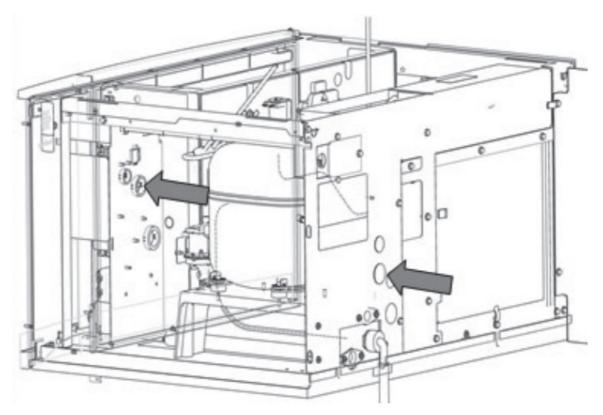
7. Connect the probe molex connector into the bin level port on the control board as shown.
