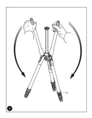
Unfold the legs as shown in fig. 1
