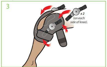
Position the compression garment on the leg so knee cap appears in the opening. Apply a hinge assembly on each side of the knee with the hook attachment. Center the hinge with the knee joint. The uprights should be aligned with the middle of the leg. Wrap hook and loop straps to secure in place.
