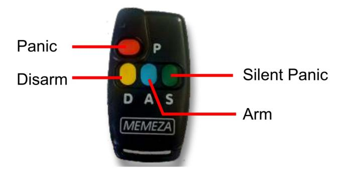
Pressing Panic will trigger the siren output and the onboard buzzer will beep for 2minutes, device to transmit Panic to cloud Silent Panic will make not audible noise and transmit a Duress Panic to the cloud. Arm is indicated by a single beep. 30 seconds is given as an exit delay. Disarm is indicated by 2 beeps After any alarm or panic activation the siren and onboard buzzer can be silenced by pressing the disarm button
