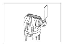
When using sanding application tool, mount the application tool on the sanding pad so that it matches the sanding pad direction.
