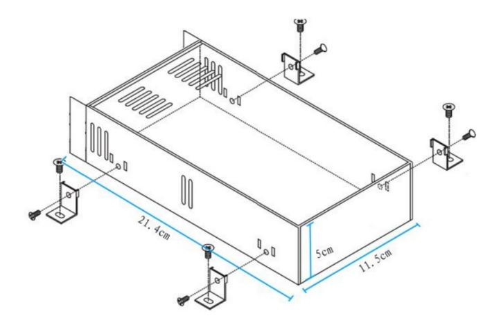
**Notes:** Please use our screws only since it may damage the internal PCB if using other screws. Please use proper torque to push the screws into casing since it may damage the internal PCB by strong torque. **Content Included**
