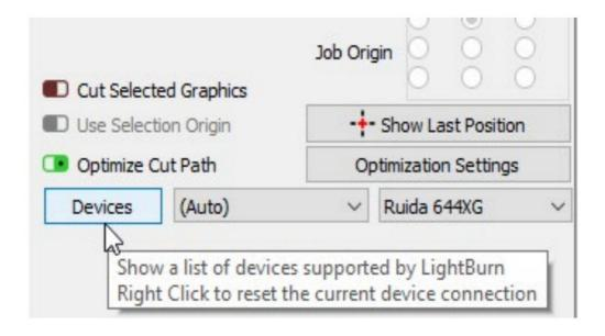
LightBurn can also be configured to control more than one laser, and there are settings stored for each device. If you don't pick one, we have nowhere to put these settings, and a number of features within LightBurn will not work until this is set up.
