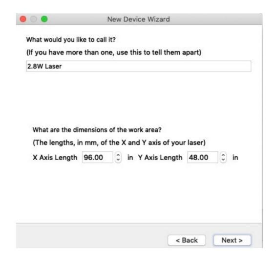
You must set the size of the work area for your laser so that LightBurn can make try to prevent things from going out of bounds. If you don't know the exact size, you can easily change this later on the Device Settings page.
