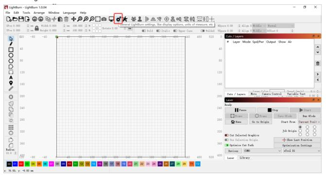
2. Enable Show rotary enable on main window in the Settings window that appears, and click OK.
