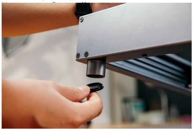
2. Fit the rubber ring to each cylindrical spacer block.
