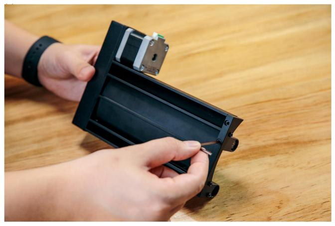
2. Pull up the support of the movable roller. Rotate the movable roller to the target position.
