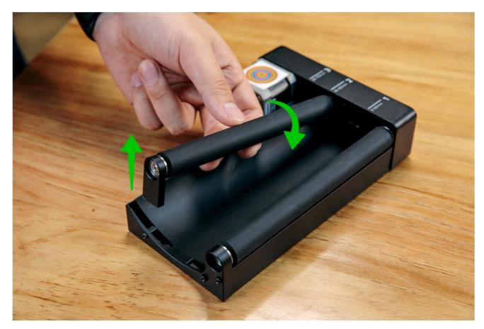
3. Put the support of the movable roller into the corresponding slot and press it into place. The side with a concave part faces away from the movable roller.
