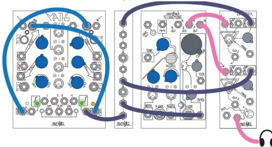
Briefly turn on MATHS Ch. 1 Cycling and wait for Ch. 4 to be triggered via EOR. At which point, press the Ch.1 CYCLE Button again in order to disengage cycling, allowing the trigger loop to continue indefinitely.
