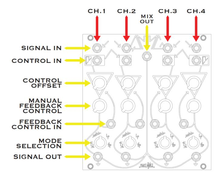
The QMMG is comprised of 4 identical channels each having the following:
