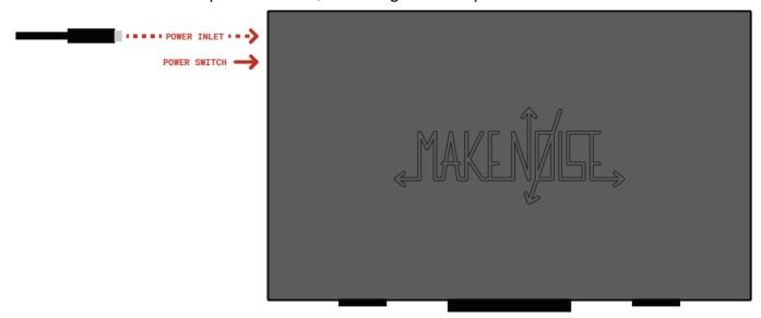
The plug has a sliding sleeve. To remove the plug, slide the sleeve away from the case, and gently pull on the plug. It should come away easily.
