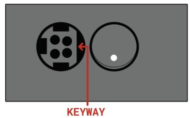
To install the adapter, place the case on a flat surface with the switch and power inlet on the far left. The adapt-er plug has a 'D' shape. With the flat of the D facing away from you, insert the plug into the power inlet. The plug should lock into place. This locking feature is useful for live performance, ensuring that the power remains connected.
