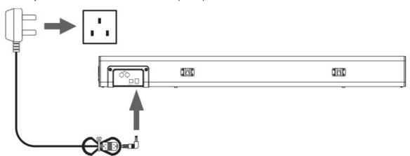
Ensure all audio connections of the unit are connected before connecting to the mains power socket. Unplug the power cord from the outlet when the unit is used for an extended period of time.
