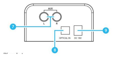
7. AUX socket 8. OPTICAL IN socket 9. DC IN (18V) socket
