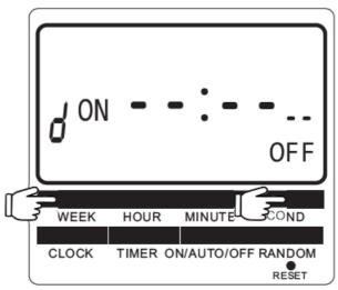
You can press "HOUR", "MINUTE" and "SECOND" to set the count down time you want, the duration of count down can be set from 1s to 99h 59m 59s.
