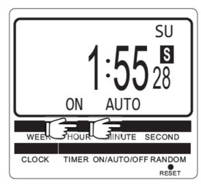
This function will allow the timer to adjust the current clock time on the timer by an hour ahead to accommodate daylight savings. Press "HOUR" and "MINUTE" again to exit the Summer Time mode
