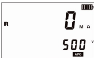
Figure 9-4 Insulation resistance measurement mode
