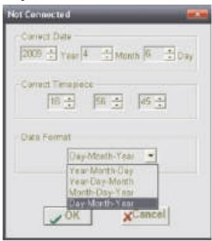
Input the correct date and correct time and select the date format display on the Data Logger , and click "OK" button then Data Logger time will update.
