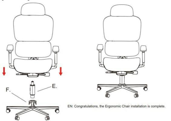
6. Assembling the Ergonomic Chair with gas lift, seat and legs together
