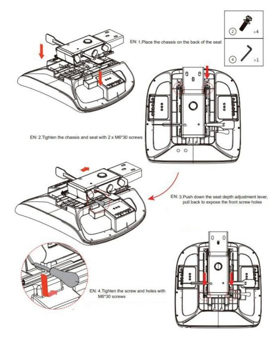
1. Installation of seat and chassis
