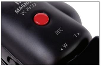
2. Use the variable-speed zoom rocker switch to control the zoom function.
