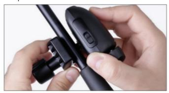
4. Place the controller on the panhandle, with the handle centered in the clamp's V shape.
