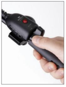
3. Press the side of the switch marked "W" to zoom out to a more wide-angle view; press the "T" side to zoom into a more telephoto view.
