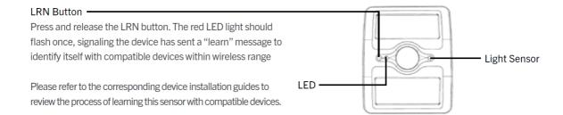
NOTE: It is recommended that pairing of device be done prior to installing the ceiling sensor
