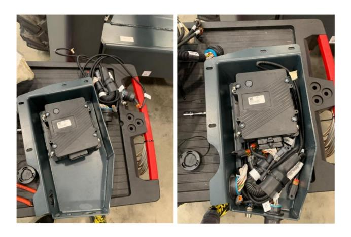
• Secure the CTB-D connector to the cover and seal it with the provided cap.
