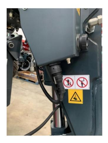
• Attach the attachments recognition sensor (cod. 113519) to the bracket (cod. 113520) maintaining a distance of 3 cm and tighten the sensor's locknut to ensure a secure fit.
