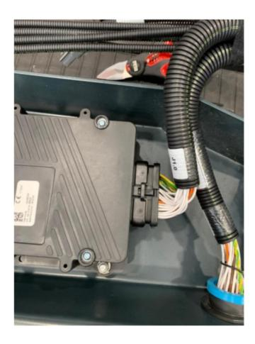
• Secure the ANT-2 connector plug to the cover, which will be used for connecting the new attachments recognition sensor.
