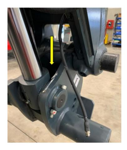
• Install the new attachments recognition sensor by securing the bracket on top of the boom and connecting the cable to the wiring connector inside the cover.
