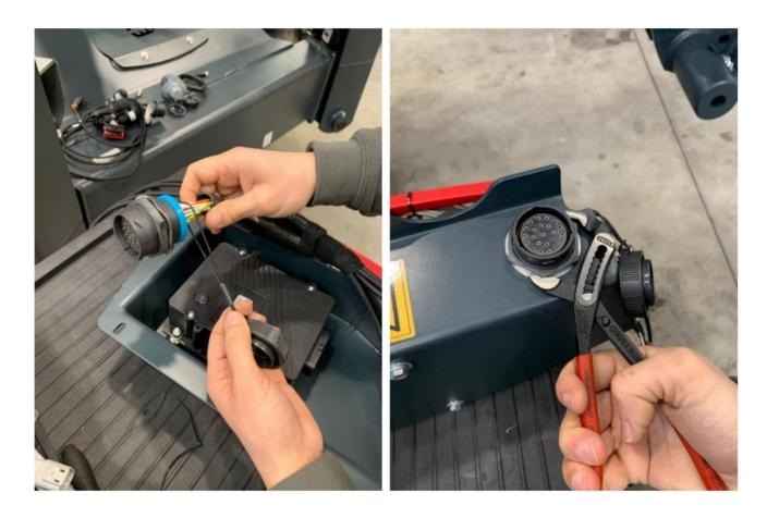
• Connect the J1.0 connector to the Boom ecu.
