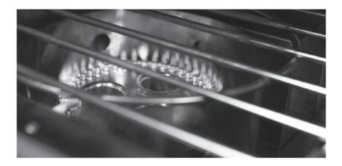
Normal flame should be all blue and look like it's touching the burner at the bottom, with a minimal amount of yellow/orange.
