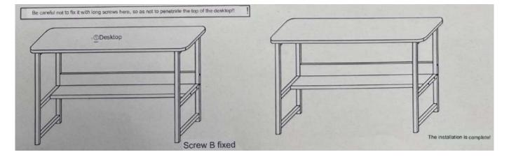
Be careful not to fix it with long screws here, so as not to penetrate the top of the desktop! The installation is complete!
