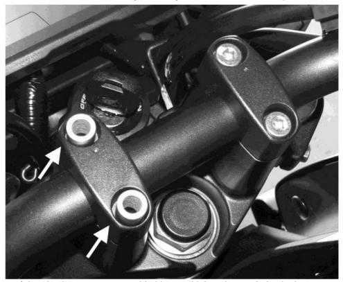
STEP 2- Set two of the aluminum spacers provided in your kit into the two holes in the now-open top clamp, as seen in the photo above. Put one M8 flat metal washer on top of each spacer. To keep it from slipping off, put a dab of Vaseline or similar thick grease on top of the spacer so that the flat washer will stick to it and not slide off.
