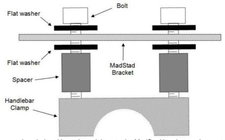
Or, pre-assemble the new long bolts with washers right onto the MadStad bracket as shown at right.
