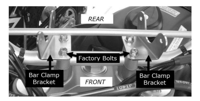
STEP 2 – Run the two factory bolts through the Bar Clamp Bracket for that side (see photo above) and add two flat washers. (See hardware diagram below).
