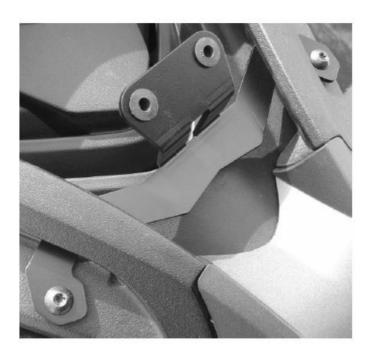
To keep the metal arms of the bracket from laying directly on the metal of the bike we have provided two "shoulder washers" to sit between the two (see photo below). The shoulder washer has a raised centre and a wide rim. The wider portion is the top. Run the screw through the front bracket then the shoulder washer then into the mounting hole, as in the diagram below. If the factory screw is too short for any reason, use the M5 x 45mm Phillips screws provided in your hardware kit.
