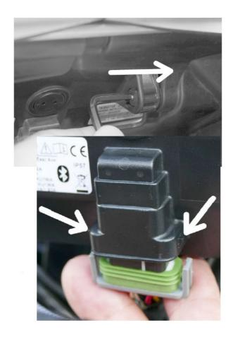
Once the panel comes free from the housing, unplug the cable from the back. There are two snap posts under the U-shaped gray retainer (one on each side) so you will need to pry that retainer off on both sides to release the plug (see image at right).
