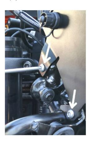
Once the electrical components are installed, set the assembly over the four OEM threaded frame mounting holes that the original plastic housing was on, and screw the assembly on with the original four housing screws. (See photo at right). Make sure these screws are all tight.
