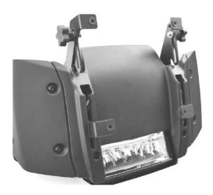
Before attaching the windshield, check the adjustable brackets and make sure they are in the same position of height and angle. If not then loosen the knobs one turn to change height, and several turns to release the angle adjustment so you can set both in the same position. See the "Adjusting the Brackets" section on the next page for details.
