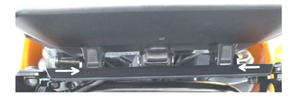
Insert the M5  $\times$  35 Phillips screws in each side and screw them in until snug. Take care not to push hard on the screwdriver, you could push the well nut out of the other side.
