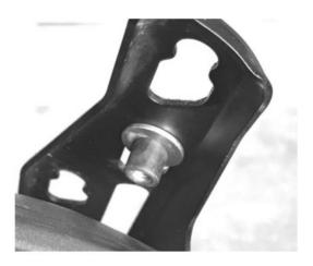
Once the well nuts are in place you can attach the MadStad brackets as shown here by using the factory windshield screws. Do not overtighten the screws; they should be snug and tight but do not crank down hard, that could damage the well nuts. As long as they swell up behind the D-washers they will not come out.
