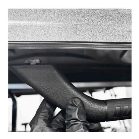
**STEP 2** Align the 'T' nuts with the inside wide track as shown.
