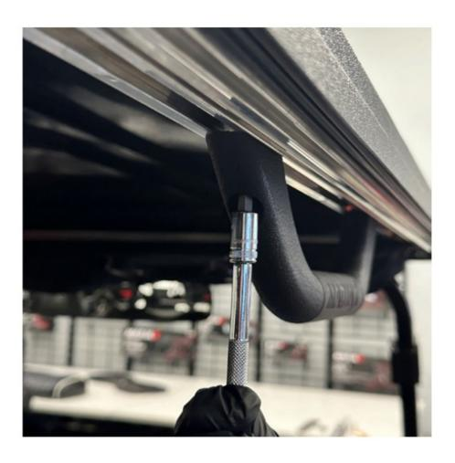
**STEP 4**Tighten the allen head hand tight to ensure the grab handle is secure to the top and use supplied plugs to cover bolt holes.
