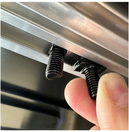
**STEP 2**Place grab handle mounting bracket onto the 'T' studs with the flat side facing out, as shown in Step 3.
