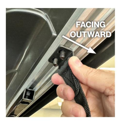
**STEP 4**Using a 13mm socket, hand-tighten down the locknut securely, ensuring the 'T' stud is fully engaged with the track.
