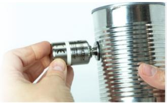
7. Screw the HiTemp140-CF into the ThermaLock until the threads are no longer visible. This will compress the black fer rule creating a hermetic seal
