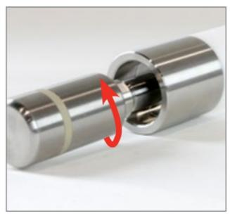
4. Slide the probe of the data logger out from the lid of the thermal barrier.
