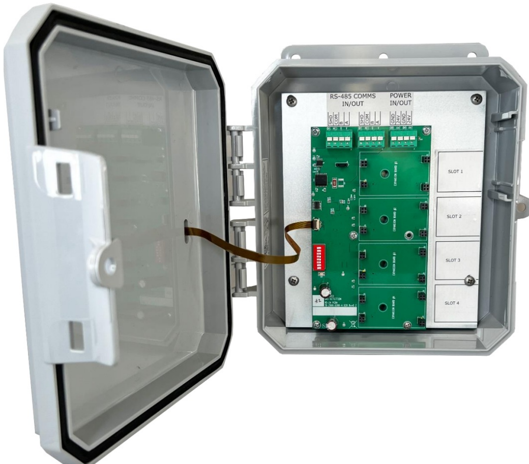
Figure 3-2 – Internal view with expansion boards
